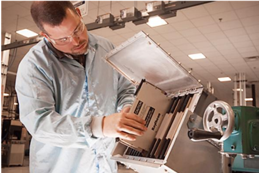
3. A modular, board-level approach to the design and construction of large radar systems can simplify repair and maintenance. (Photo courtesy of Raytheon Co.)
