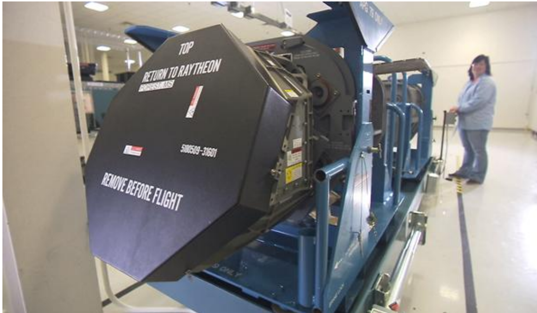
2. The AESA radar is a multimode radar system that has been installed in a large number of F-15 fighter jets throughout the world. (Photo courtesy of Raytheon Co.)
